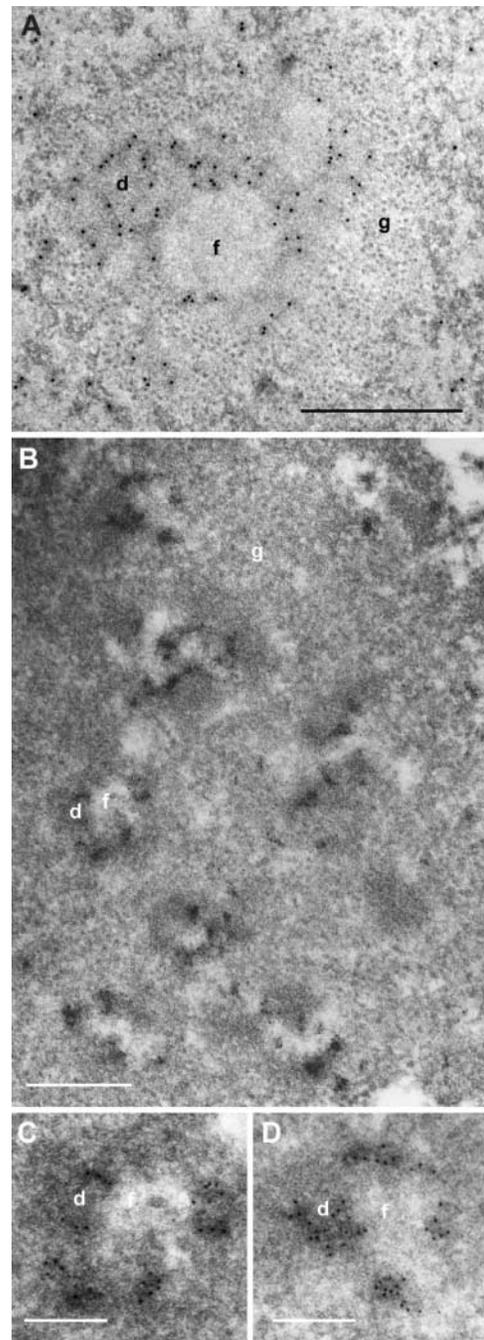
**Figure 3. EM mapping of nucleolar transcription in HeLa cells.** (A) Nucleolar EM transcription signal observed in hypotonically treated cells is confined to the DFC. (B–D) EM localization of transcription in thin-sectioned permeabilized cell. (C and D) Detailed parts of B. Nucleolar transcription signal consists of numerous clusters of gold particles accumulated in the DFC. (A) Bars: 0.2  $\mu\text{m}$ ; (B–D) 0.5  $\mu\text{m}$ .
